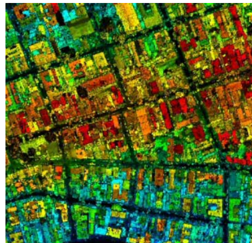
Fig. 6 View from the top of point cloud through hypsometric color representation.
