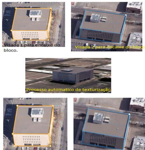
Fig. 17 Example of docking blocks in building and texturing process automatic.
