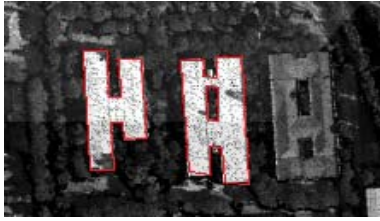
Fig. 11 In red, the automatically generated vector created from the points related to the buildings.
