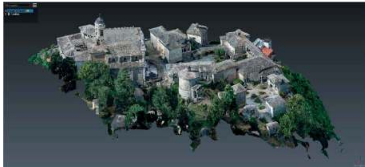
Final point cloud obtained by the UAVs survey. Top view of the Piazza del Tempio and Piazza dei Tribunali
