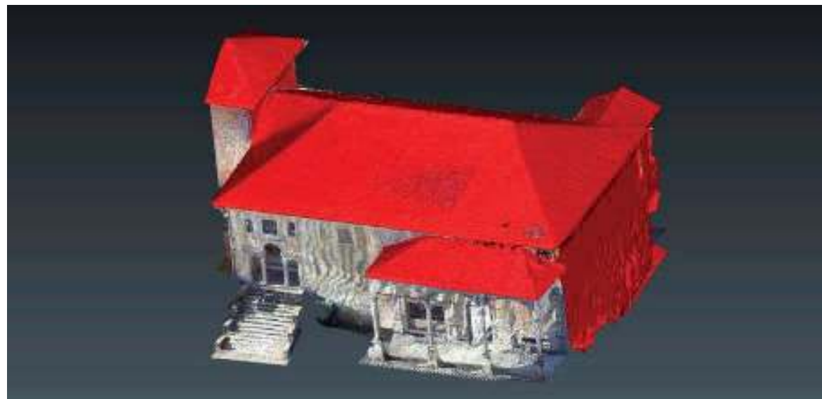
Overall point cloud of the Palazzo di Pilato. Red colored the parts taken from the UAVs survey, the remaining parts come from the LiDAR survey.
